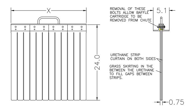
CHUTE BAFFLES ARE MADE TO ORDER BASED ON WIDTH REQUIRED FOR THE APPLICATION. WHEN ORDERING PLEASE SPECIFY DIMENSION "X" IN THE DIAGRAM ABOVE
