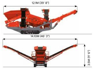
MACHINE WEIGHT: 18,300KG (40,350LBS) WITH BELT FEEDER
