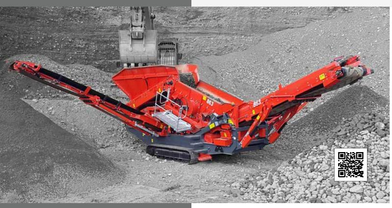
The Finlay<sup>®</sup> 863+ mobile scalper is a compact and aggressive forward facing screen. This flexible and mobile plant can work in aggregates, sand and gravel, top soil, construction demolition and recycling applications where site space is at a premium.
