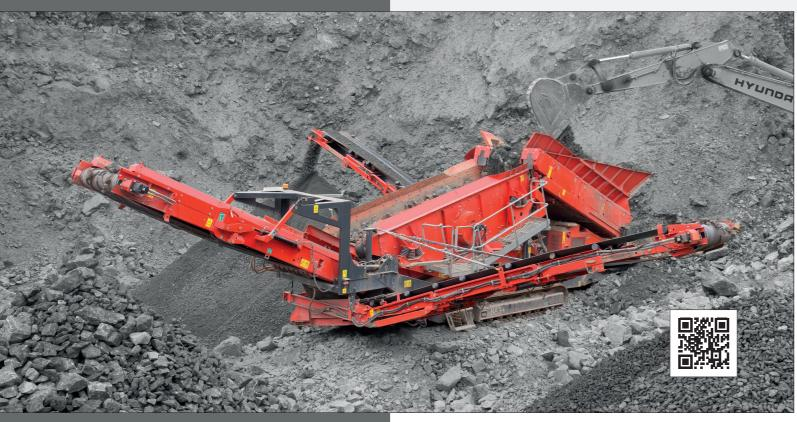
The Finlay® 883+ mobile scalping screener has been developed as a high capacity and versatile heavy duty screener to work in primary and secondary screening applications such as quarry and mining, iron ore, construction demolition waste, sand, gravel, compost, top soil and coal.
