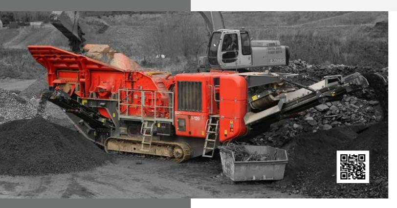
The Finlay<sup>®</sup> I-120 mobile impact crusher has been designed with improved material flow and enhanced productivity in quarrying, mining, recycling and construction demolition applications.
