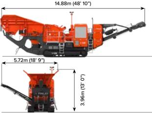
MACHINE WEIGHT: 37,000kg (81,571lbs) (Pre-screen, Hopper Extensions, By-pass Conveyor & Twin Pole Magnet)
