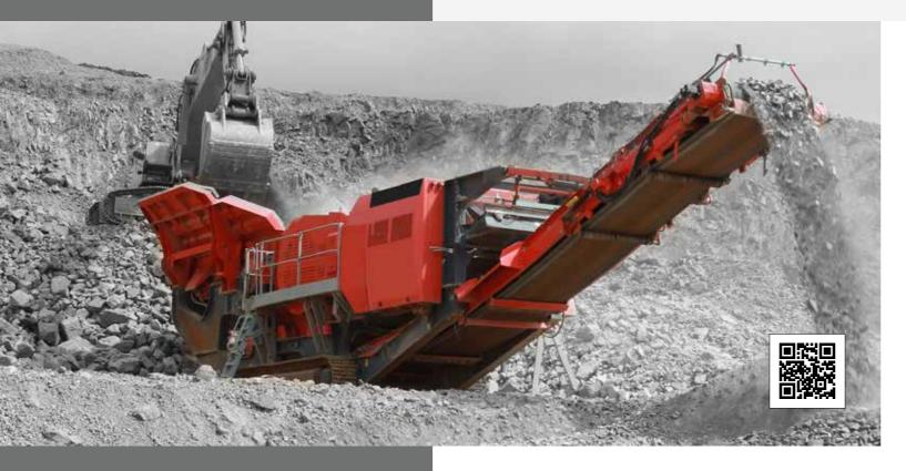
The Finlay<sup>®</sup> J-1480 incorporates the Terex Jaques JW55 single toggle jaw crusher which boasts a throughput capacity up to 750mtph depending on application and material.
